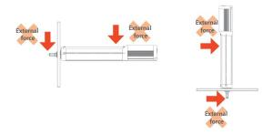
When using front bracket mounting, flange (front) mounting, etc., if the device is mounted horizontally, secured at a single point, and has a stroke of 150mm or more, prepare a support block as shown in the figure below even if there is no external force applied on the body.
