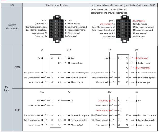
(Note 1) Switching to the single solenoid method will change B3 to "forward/backward command" and B4 to "unused."
